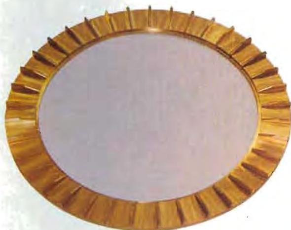
Figure 4. The single solid-cast separator ring.
